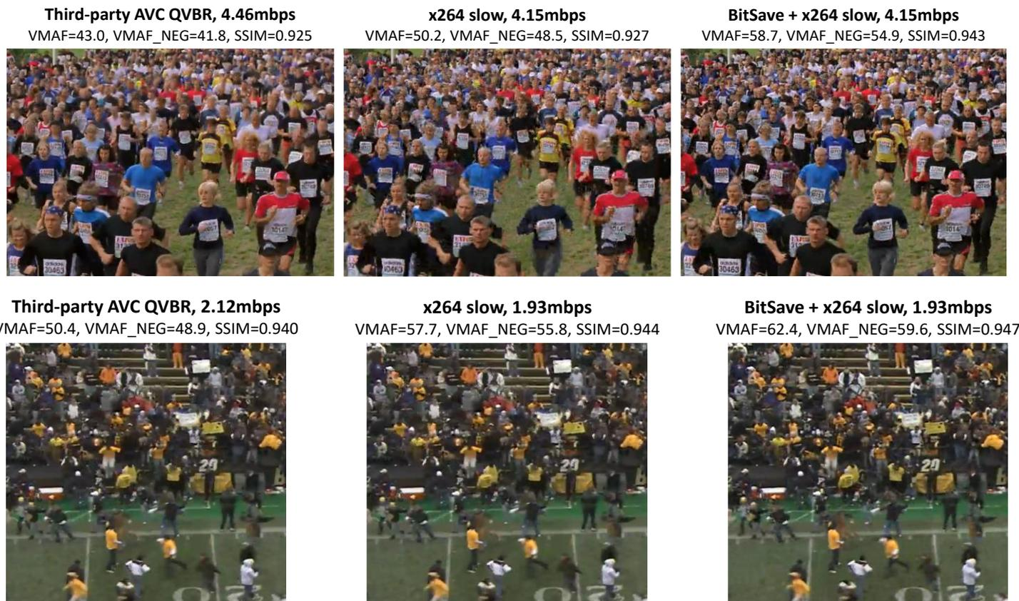
Figure 3. Visual comparison of encodings corresponding to Table 1 (top: 'crowd run'; bottom: 'rush field cuts'). x264 and BitSave + x264 is at approx. 8% lower bitrate than the third-party AVC QVBR.
